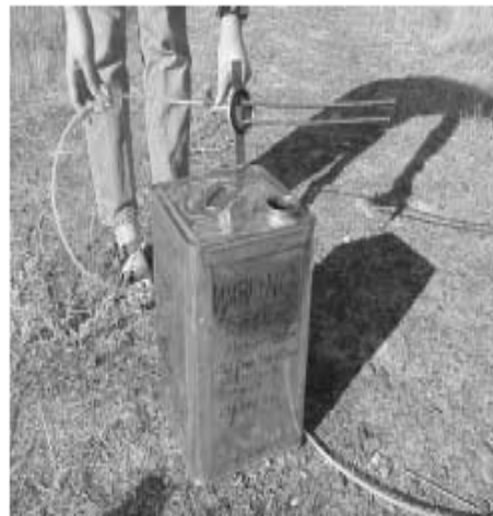
Figure 3.4b Close up showing plumbing of continuous drip can. (Note: This can is empty. Appropriate safety gear must be worn when applying rotenone.)
