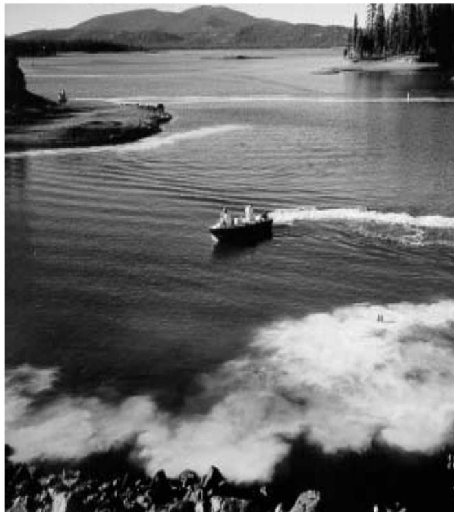
Figure 3.1c Liquid rotenone dispersion using a boat with a holding tank and boat bailer system. Lower figure shows rotenone being dispensed with this equipment.
